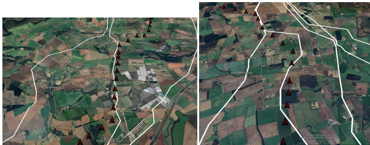
Examples of TKUP oblique crossings, close proximity and parallel courses. Monboddio & Cullerie areas (Pipelines=White)
